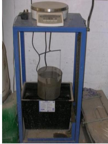
Figure 4. Density testing apparatus (weight-in-air/weight-in-water method)
